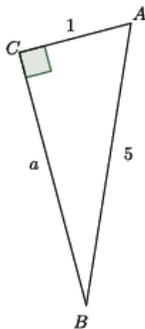
$$\begin{aligned} a^2 + 1^2 &= 5^2 \\ a^2 + 1^2 - 1^2 &= 5^2 - 1^2 \\ a^2 &= 5^2 - 1^2 \\ a^2 &= 25 - 1 \\ a^2 &= 24 \end{aligned}$$
