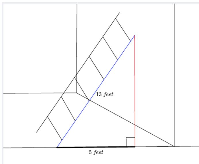
The ladder against the wall forms a right angle. For that reason, we can use the Pythagorean theorem to find out how far up the wall the ladder will reach. If we let  $h$  represent the height the ladder can reach, what equation will represent this problem?
