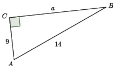
$$\begin{aligned} a^2 + 9^2 &= 14^2 \\ a^2 + 9^2 - 9^2 &= 14^2 - 9^2 \\ a^2 &= 14^2 - 9^2 \\ a^2 &= 196 - 81 \\ a^2 &= 115 \end{aligned}$$
